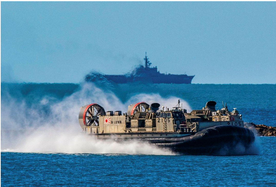
An air cushioned landing craft launched from the transport ship JS KUNISAKI (2019) (Source: Australian Department of Defence)
